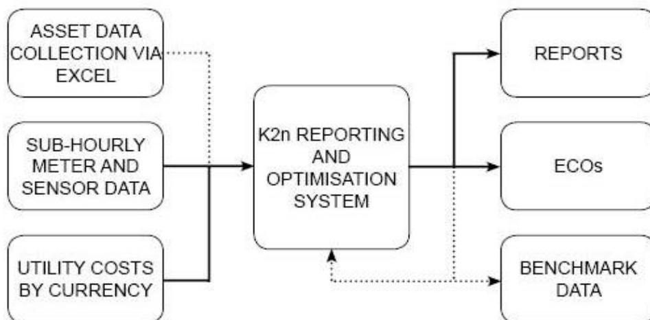
The K2n National Database helps enable continuous improvement in schools energy and water performance based on potential savings identified by the collection and analysis of sub-hourly energy and water end use data. It monitors plant performance related to different activity areas and compares the performance to benchmark data for that relationship. It can be used by the School and/or contractor to identify Energy Conservation Opportunities (ECOs).
